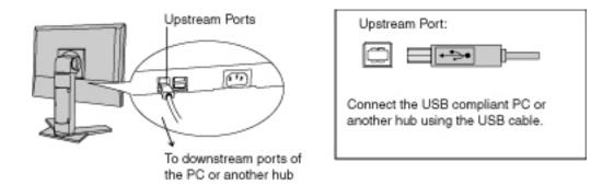
After connecting the USB cable, the USB function can be set up automatically.
